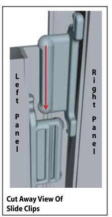
Components connect together by aligning them and sliding downward connecting clips together.
