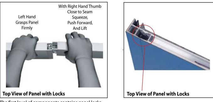
The first level of components contains panel locks that are located at the top of the panel for extra stability and a seamless connection. When disassembling panels, twist top connection slightly and lift right panel upward.
